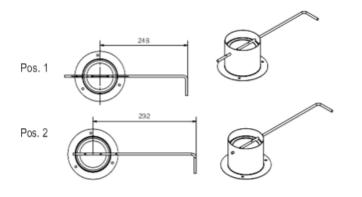
• Adjust the operating leaver of the connecting piece in accordance with the table and depending on the stove model.
