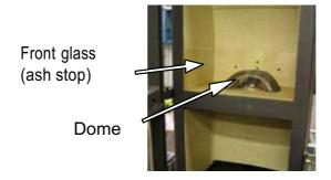
Regarding the cleaning of the upper combustion chamber the ash pan can be used. The pan is placed underneath the UCC in 2 brackets.
